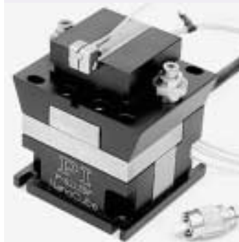
NanoCube™. Compact XYZ NanoAlignment system with 100 µm travel range in each axis and 1 nm resolution, shown here with the F-603.22 fiber-holder ferrule. For more information on this product, see pages 2-36 and 9-18 in our 2001 catalog or visit www.pi.ws
