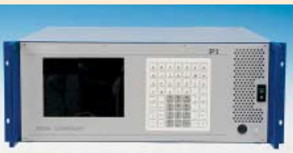
Reliable control of all 273 axes is based on 9 custom PI C-880 multi-axis automation controllers with custom interfacing, firmware and software.
