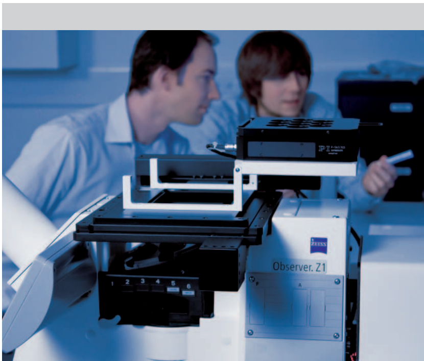
Novel laser lithography system which – for the first time – allows the production of complex three-dimensional microstructures and nanostructures using photosensitive materials. The precise adjustment of object or sample is achieved by using a P-563 PIMars™, a parallel-kinematics multi-axis piezo nanopositioning system (Photo: Nanoscribe)
