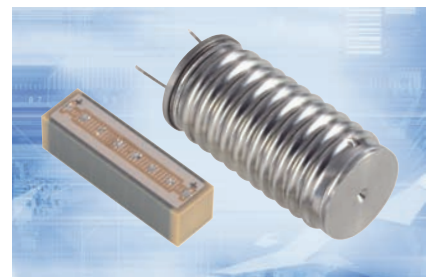
Two PICMA ® piezo actuator versions (5 x 5 x 18 mm ceramic type): Conventional multilayer actuator and actuator with a hermetically sealed stainless steel casing
