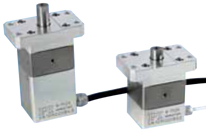
N-111 NEXLINE ® Piezo stepping drives: high resolution, large travel and heavy loads. Piezo stepping drives combine piezo actuators with different motion characteristics. When driven in an appropriate way, both clamping and driving motions can be realized, the latter resembling the motion of a quadruped.
