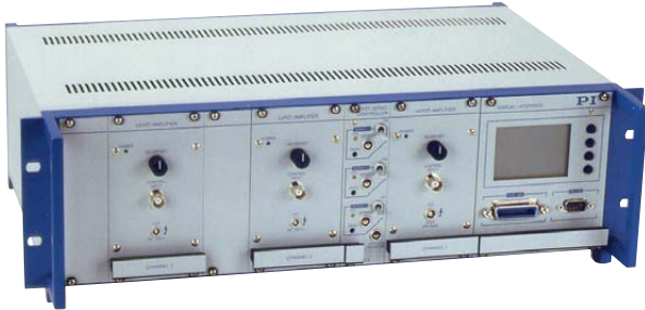
Configuration example: E-500 chassis with three optional E-507 HVPZT amplifiers, E-509.L3 piezo servo-controller for LVDT sensors and E-516.i3 20-bit DAC interface/display.
