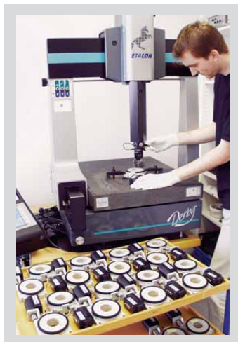
Custom M-038 stages at the coordinate measuring machine
