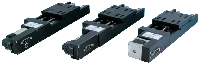
Different motor versions of the M-403 linear stage family with 100 mm travel range (from left): M-403.4PD (DC-motor/ActiveDrive™), M-403.4DG (DC-motor/gearhead) and M-403.42S (stepper motor).
