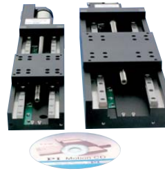
Profile comparison between M-403/M-404 (left side) and M-413/M-414, which was designed for higher load and travel ranges.
