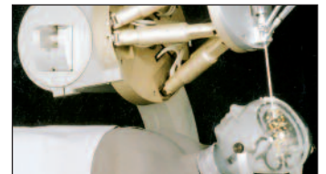
Custom Hexapod designed for neurosurgery Photo: IPA
