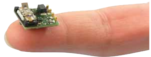
The P-653 miniature drive including the drive electronics measures only 11 mm
