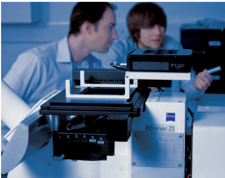
Novel laser lithography system which – for the first time – allows the production of complex three-dimensional microstructures and nanostructures using photosensitive materials. The precise adjustment of object or sample is achieved by using a P-563 PIMars™, a parallel-kinematics multi-axis piezo nanopositioning system (Photo: Nanoscribe)
