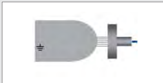
Fig. 17: Curved surfaces lead to an averaged distance measurement
