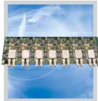
Custom, 7-channel, capacitive position sensor electronics
