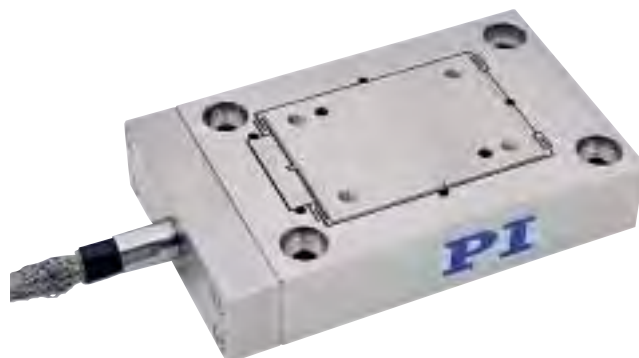
The P-752.11C piezo nanopositioning system with integrated capacitive sensors provides position resolution down to 0.1 nm
