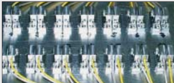
Quality control and long-term stability testing of capacitive displacement sensors at PI
