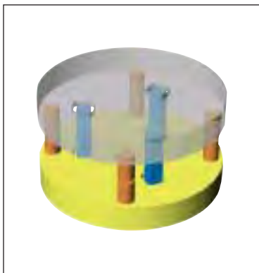
Basic design of an active optics platform featuring three actuators and four sensors
