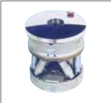
Active tip/tilt mirror for the United Kingdom infrared telescope (UKIRT) on Mauna Kea, Hawaii with Hexapod 6-D alignment system (for information on Hexapod systems, see the "Hexapods / Micropositioning" section). Mirror diameter: 314 mm Tip/tilt range: \pm 500 \mu\text{rad} Resonant frequency: 280 Hz
