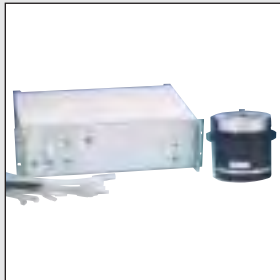
Custom tip/tilt mirror system with controllers for the Subaru telescope.
