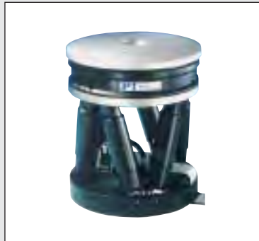
Active secondary mirror for NASA Infrared Telescope Facility (IRTF) on Mauna Kea, Hawaii, with Hexapod 6-D alignment system (for information on Hexapod systems, see the "Hexapods / Micropositioning" section). Mirror diameter: 244 mm Tip/tilt range: \pm 250 \mu\text{rad} Resonant frequency: 490 Hz
