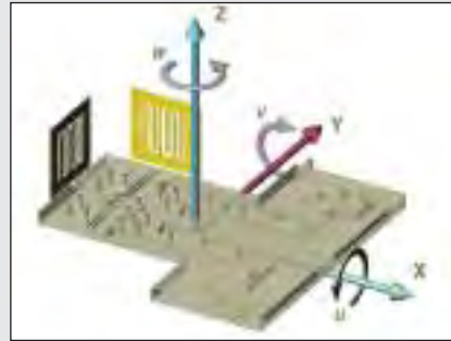
The Hexapod controller permits placing the center of rotation anywhere in space, for example, at the beam waist of a laser diode, the tip of an optical fiber or on the optical axis of a fiber array, thus greatly simplifying alignment algorithms.
