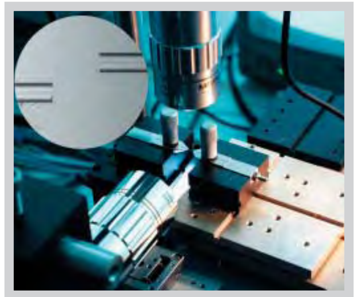
Optical fiber-alignment with F-206 6-axis-alignment system and P-611 NanoCube® 3D piezo nanopositioning / scanning system. Two cameras allow a 3-dimensional visual automated coarse alignment.
