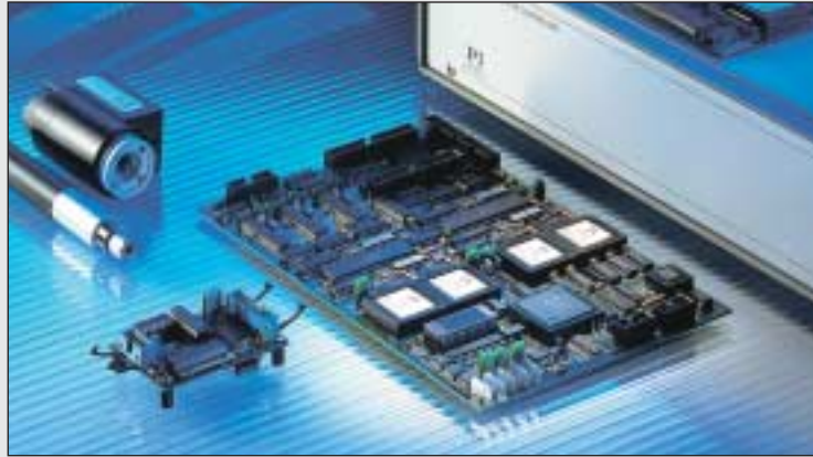
Custom 8-axis motor control card (right) and miniature single-axis controller (left).
