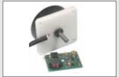
Custom rotary piezomotor with OEM driver electronics.
