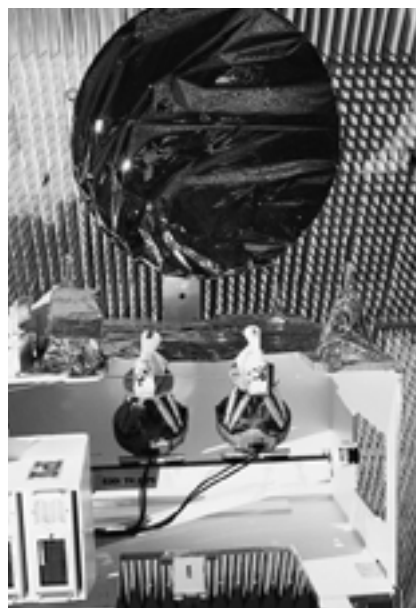
Fig. 1, Two M-850 Hexapods at Alcatel Space, Compact Antenna Test Range. This example shows optimization of the Eutelsat W4 Africa Antenna. Courtesy of Alcatel Space.
