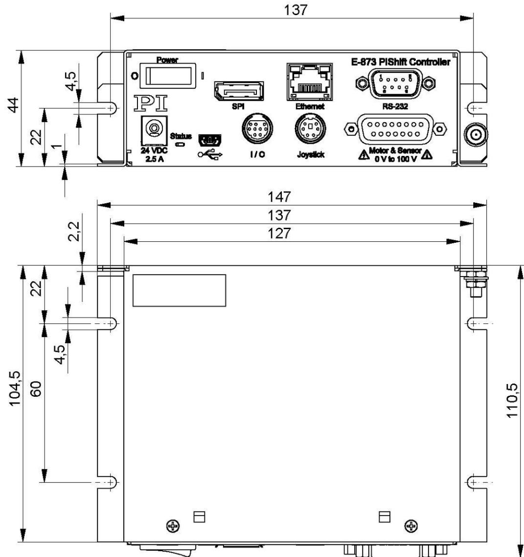
E-873.1AT, dimensions in mm. Note that a comma is used in the drawings instead of a decimal point.
