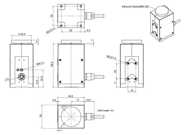
S-335.2SHM2, dimensions in mm. Note that a comma is used in the drawings instead of a decimal point. The general tolerances as specified in DIN ISO 2768-f-H are valid for all dimensions without specified tolerances.
