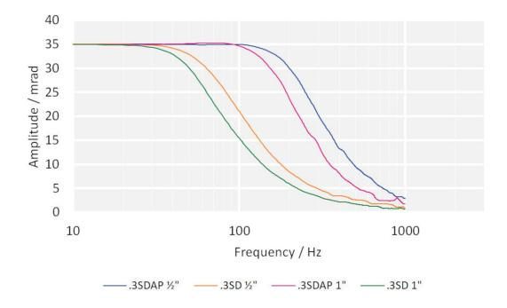
System frequency response with different E-727 controllers and mirror sizes.
