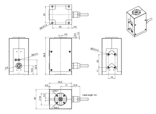
S-335.2SH, dimensions in mm. Note that a comma is used in the drawings instead of a decimal point. The general tolerances as specified in DIN ISO 2768-f-H are valid for all dimensions without specified tolerances.
