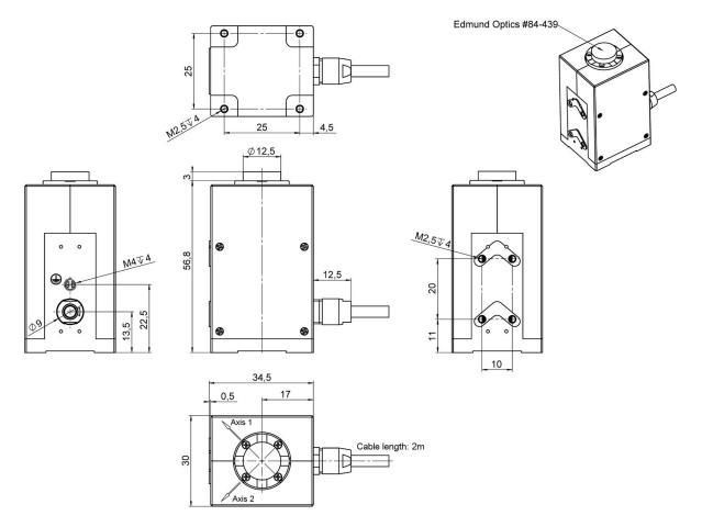
S-335.2SHM1, dimensions in mm. Note that a comma is used in the drawings instead of a decimal point. The general tolerances as specified in DIN ISO 2768-f-H are valid for all dimensions without specified tolerances.
