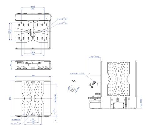
V-731, dimensions in mm. Note that a comma is used in the drawings instead of a decimal point.
