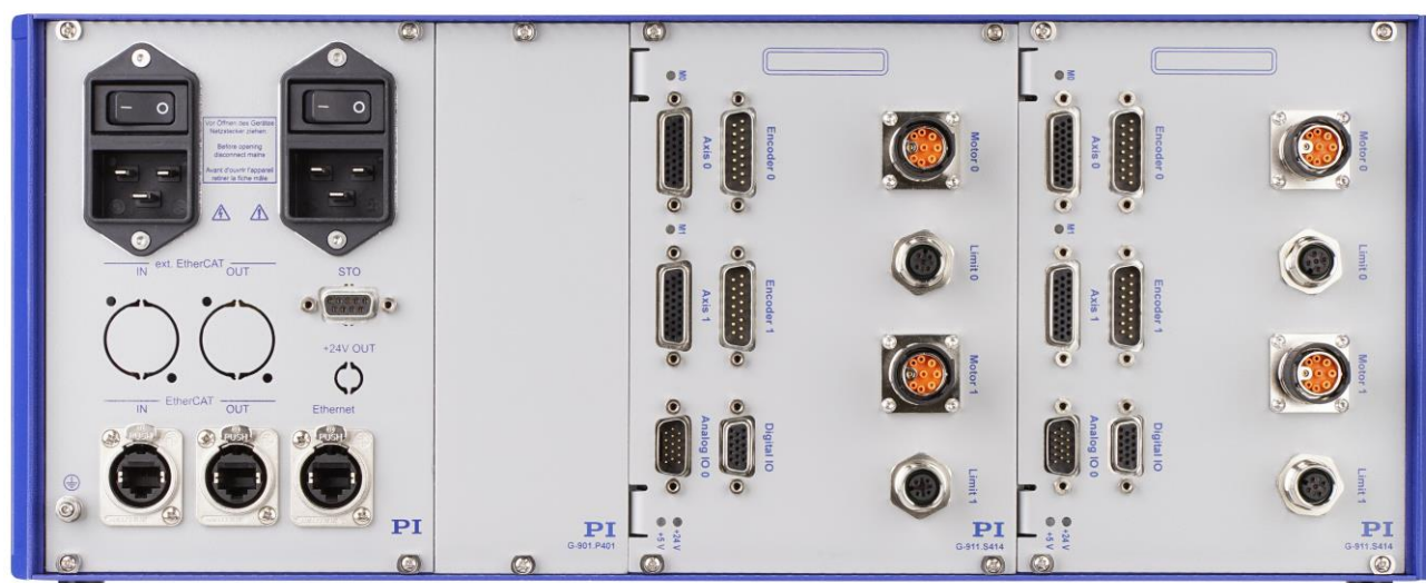
Rear panel of the G-901.R5199 with connectors
