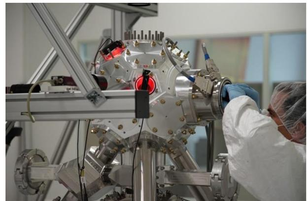
Abb. 4 Multi-axis positioning system for X-ray spectroscopy, manufactured in an ISO class 7 cleanroom at PI miCos in Eschbach, Germany
