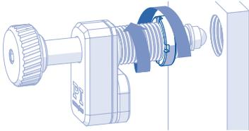
1. Screw the mounting nut in the direction of the base body.
