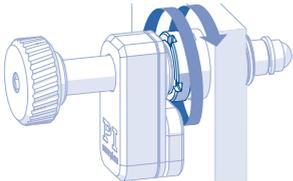
3. Hold the base body of the linear actuator and at the same time, screw the mounting nut in the direction of the mechanical mounting.
