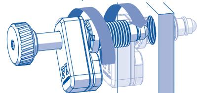
2. Screw the linear actuator as far as necessary into the threaded hole of the mechanical mounting.
