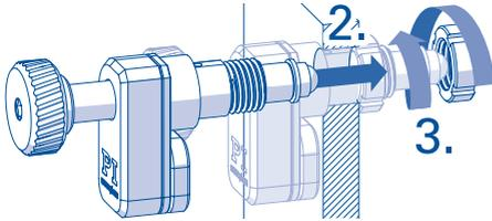
2. Position the linear actuator in the mechanical mounting.
