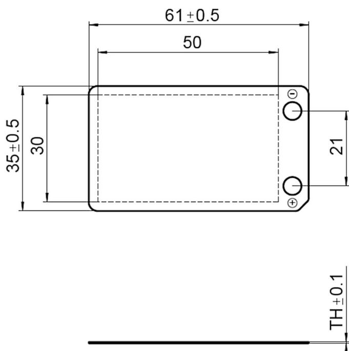
P-876.A1x, dimensions in mm. P-876.A11: TH = 0.4 mm. P-876.A12: TH = 0.5 mm. P-876.A15: TH = 0.8 mm.
