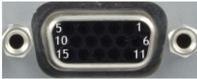
Figure 4: PZT 1...3 and PZT 4...6 HD Sub-D 15 (f) sockets on the E-135.601M drive electronics
