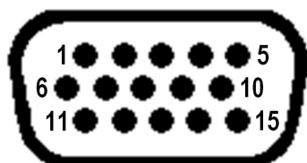
Figure 7: HD D-sub 15 motor connector (m), front view (not the soldering side)
