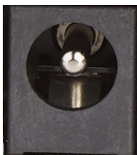
Figure 14: Power adapter connector: barrel connector socket
