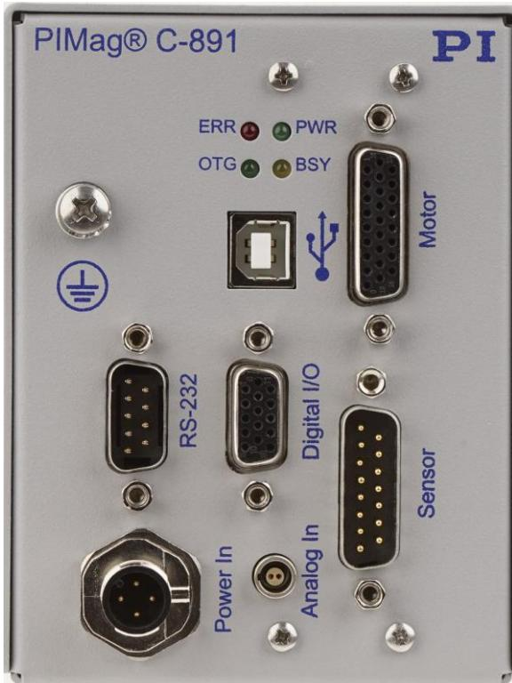
Figure 1: Front panel of C-891 PIMag® motor controller
