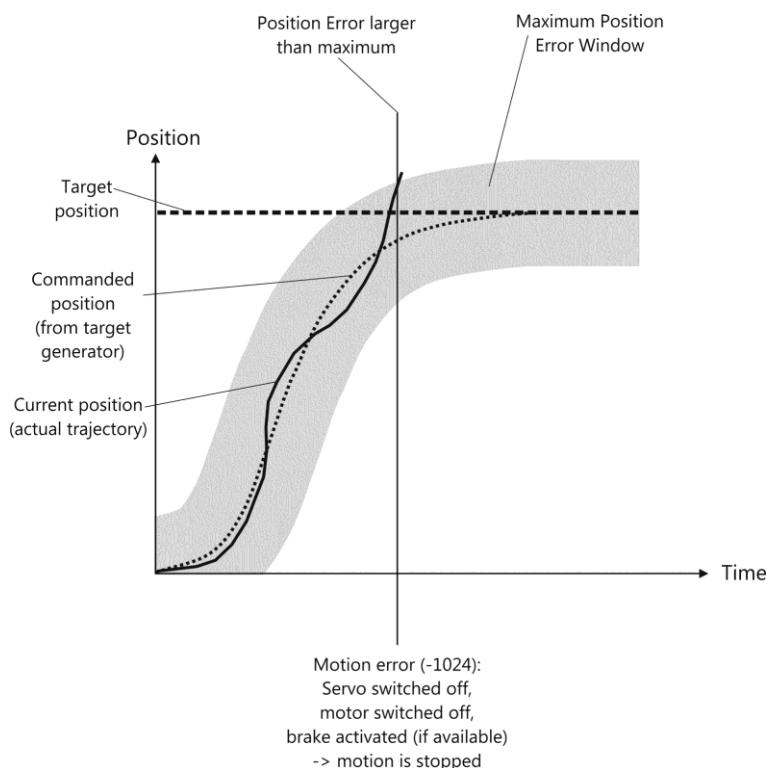
Figure 2: Behavior in case of motion errors (here, the target position was given by a MOV command)
