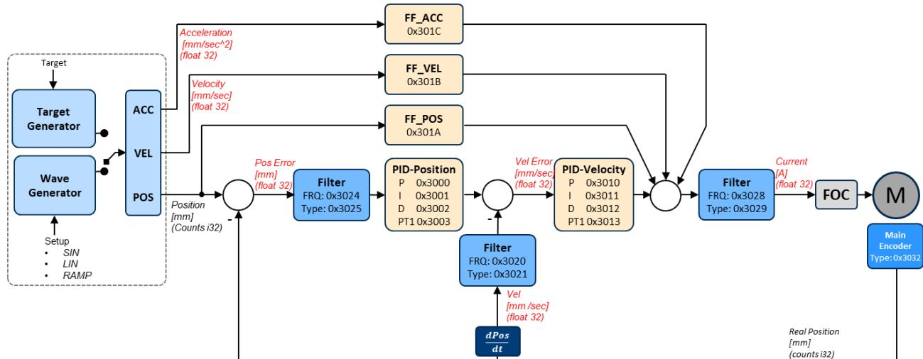
Figure 2: Alternative control algorithm: Block diagram for serial structure of position and velocity control
