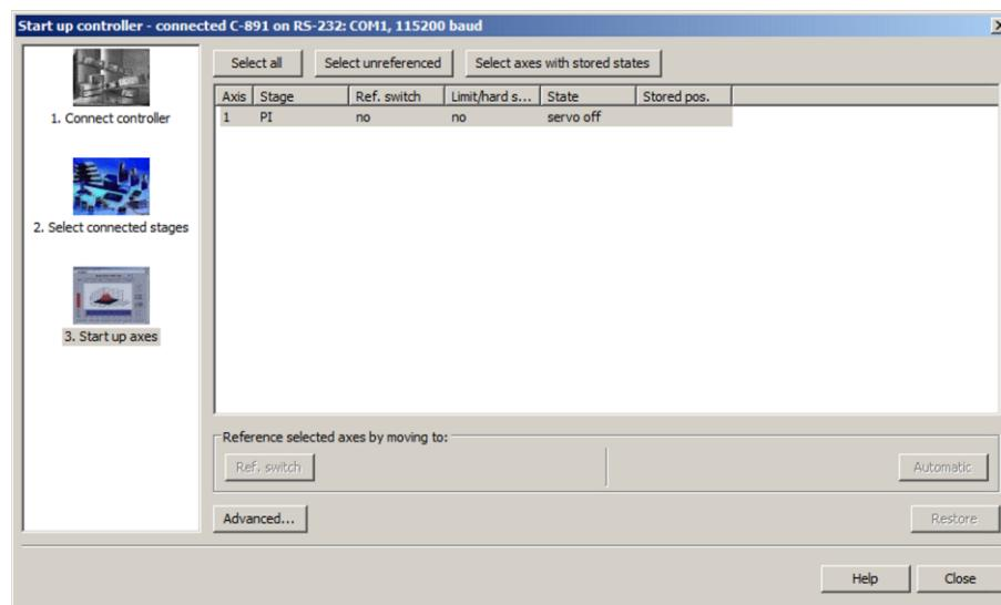
In the example shown in the figure above, a V-551 stage with absolute measuring sensor is connected to the C-891. Therefore, a reference move is **not** necessary.
