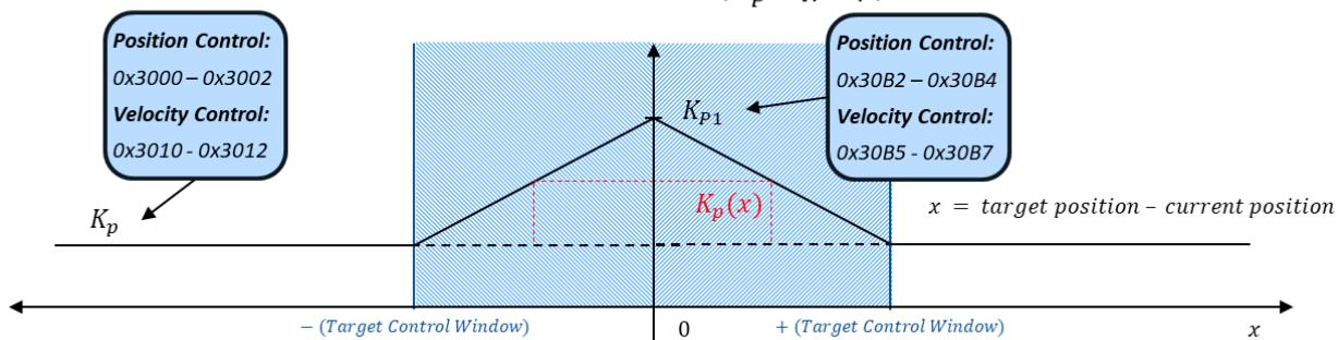
Figure 5: Adaptation of P term in the target control window; target position = 0 and  $x$  = target position – current position
