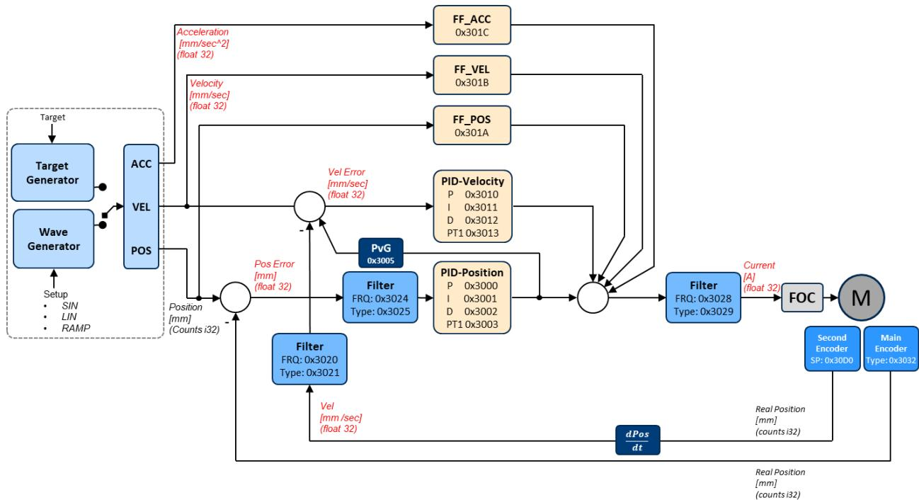
Figure 3: Control algorithm: Block diagram for parallel structure of position and velocity control with second sensor
