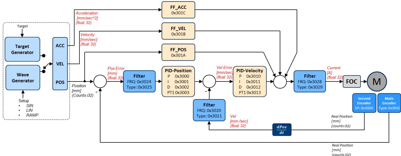
Figure 4: Alternative control algorithm: Block diagram for serial structure of position and velocity control with second sensor
