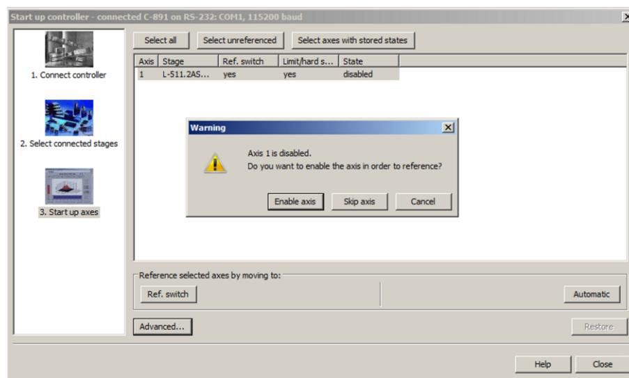
In the example shown in the figure above, an L-511 stage with incremental sensor is connected to the C-891. Therefore, a reference move is necessary.
