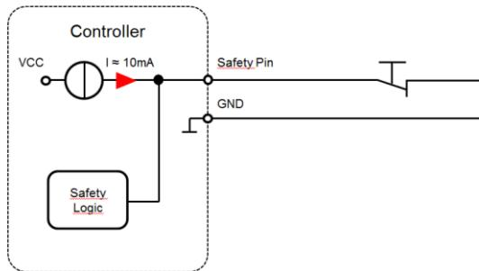
Figure 6: Signal path for connection of external hardware switch;
