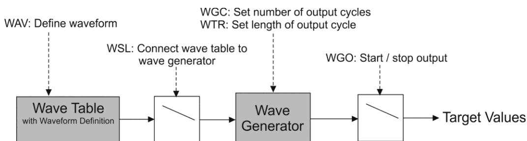
Figure 7: Block diagram of the wave generator
