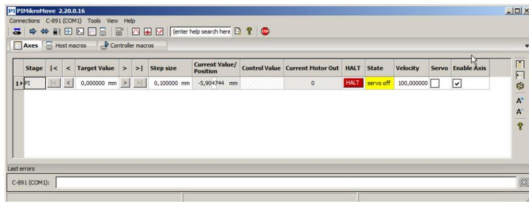
11. If the stage has an incremental or absolute measuring position sensor: On the **Axes** card in the main window of PIMikroMove, switch on the servo mode for the axis by marking the check box in the **Servo** column.
