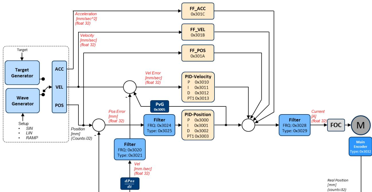
Figure 1: Default control algorithm: Block diagram for parallel structure of position and velocity control
