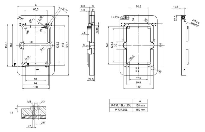
P-737, dimensions in mm. Note that a comma is used in the drawings instead of a decimal point.
