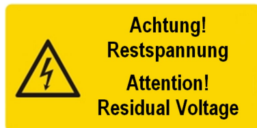
Figure 2: "Residual Voltage" warning sign on the connector of the P-753 Notice of risk of electric shock (p. 5) for models with D-sub plug connector
