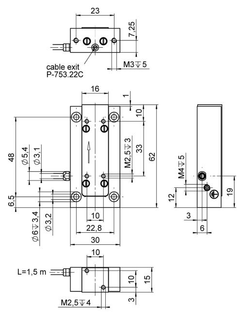
P-753.2, dimensions in mm. Max. torque at the M2.5 threads: 0.3 Nm. Note that a comma is used in the drawings instead of a decimal point.
