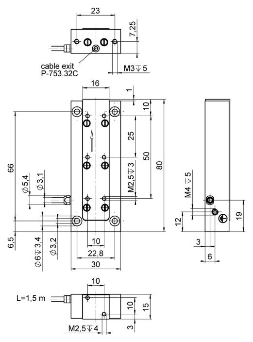
P-753.3, dimensions in mm. Max. torque at the M2.5 threads: 0.3 Nm. Note that a comma is used in the drawings instead of a decimal point.
