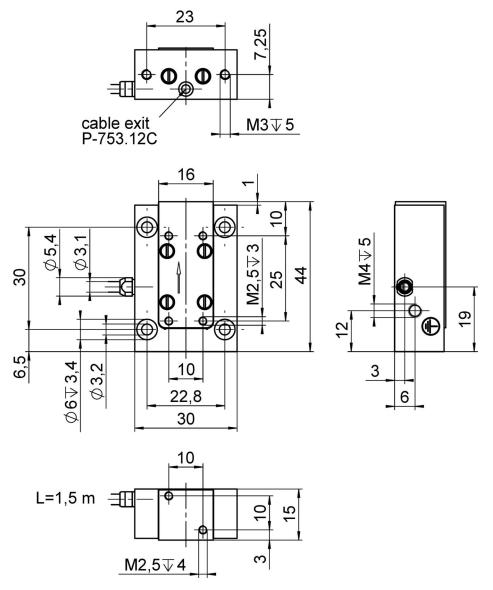
P-753.1, dimensions in mm. Max. torque at the M2.5 threads: 0.3 Nm. Note that a comma is used in the drawings instead of a decimal point.
