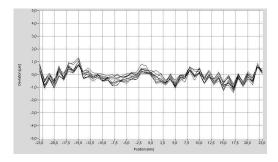
The repeatability of the M-238.5PL with linear encoder is less than 0.3  $\mu\text{m}.$
