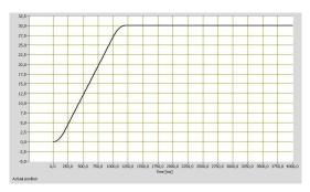
The M-238 requires less than 1.5 seconds for a 30-mm step.
