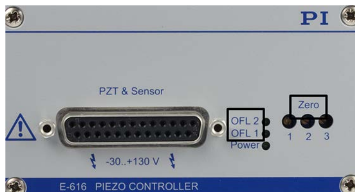
Figure 6: Potentiometer Zero 1 to Zero 3 for zero-point adjustment, and overflow LEDs
