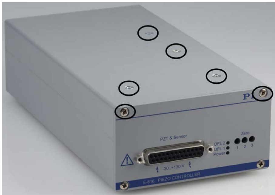
Figure 4: The top cover of the case is removed via the six labeled and two rear cross-head screws
