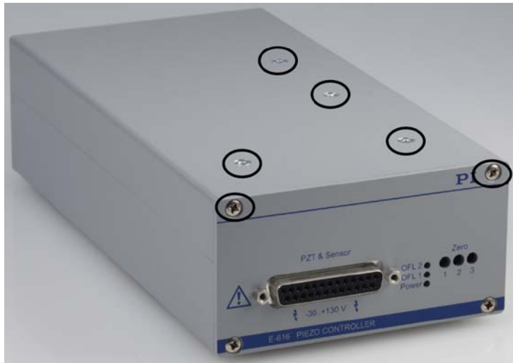
Figure 7: The top cover of the case is removed via the six labeled and two rear cross-head screws
