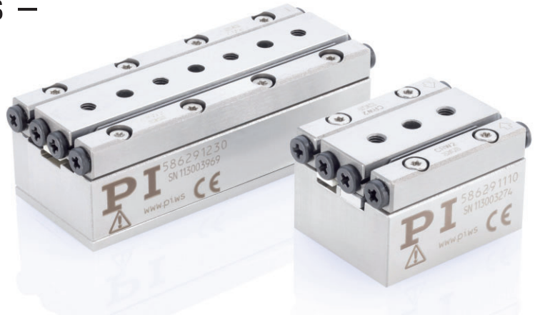
Small size and high resolution: LPS-24 miniature stages with NEXACT® piezomotors are only 24 mm wide. They achieve a 0.5 nm resolution and a minimum incremental motion of 1 nm
