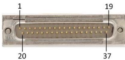
Figure 20: Sub-D 37 (m) piezo and sensor connection
