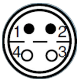
Figure 21: Sensor connector (SGS): LEMO FFA.0S.304.CLAC32Y connector, contact side
