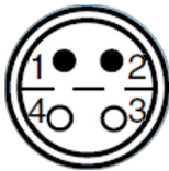
Figure 5: LEMO 4-pin connector (front view; not the soldering side)
