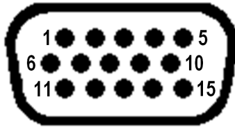
Figure 11: HD D-sub 15 connector (m) for the drive, connector side
