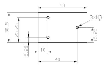
Heat sink mounting holes on top (heat sink not offered by PI)
