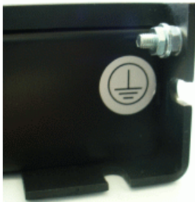
Figure 11: Where to connect the protective earth conductor (here: E-709.xRG model; E-709.CHG models have the connection on the left side of the housing)
