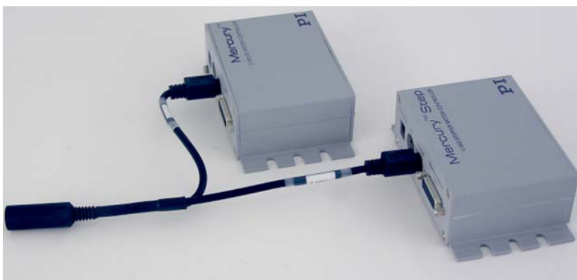
Figure 28: Y cable C-819.20Y for joystick with 2 controllers
