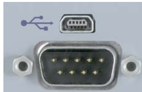
Fig. 18: Mini type-B USB connector (top) and sub-D 9-pin RS-232 (bottom)
