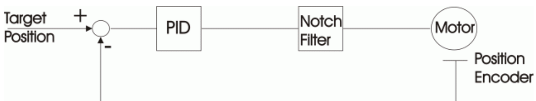
Fig. 9: Position control algorithm, with sensor feedback (position encoder in the stage) and PID correction
