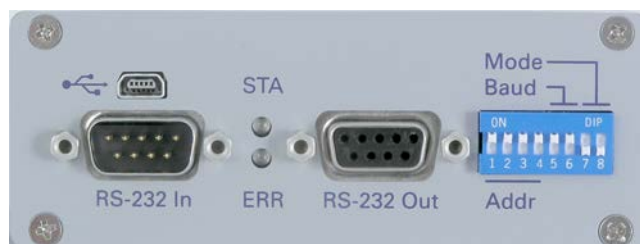
Figure 1: C-863 Mercury DC motor controller, front view
