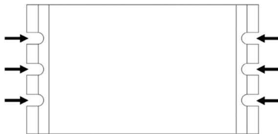
Figure 13: C-863.11: Mounting strips with recesses (see arrows)
