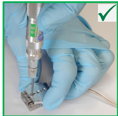
Figure 8: Correct mounting: Holding the base body and the motion platform firmly avoids torque on the motion platform
