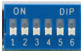
Figure 6: DIP switches 1 to 6: switch up = ON; switch down = OFF
