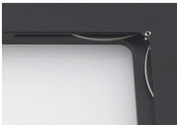
Figure 6: M-687.UO: Clip spring in aperture
