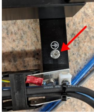
Figure 7 - Earth ground connection point location
