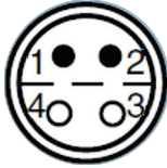
Figure 9: Sensor connector: LEMO connector FFA.0S.304.CLAC32Y, contact side
