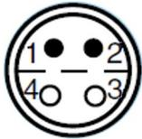
Figure 6: Sensor connector, LEMO FFA.0S.304.CLAC32, front view
