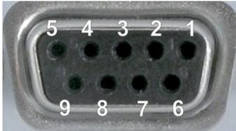
Figure 4: C-885.iD digital interface module: D-sub 9 (female)
